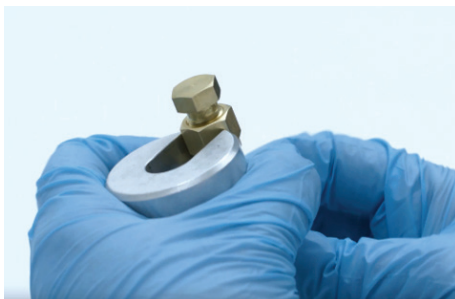
Step [9] Capping tube
