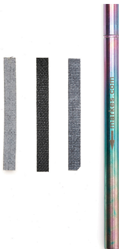
Figure 1: TF-SPME with PDMS/DVB, PDMS/CAR, PDMS/HLB and sorbent tube (left to right). PDMS not shown.
