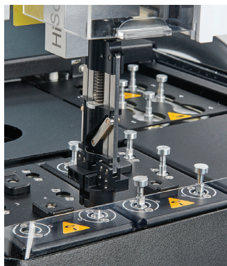
Figure 4: HiSorb probe returned to the HiSorb storage station after desorption.
