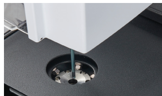
Figure 2: HiSorb probe in wash and dry station.
