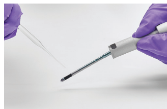
Step [4]: Rinsing the probe.
