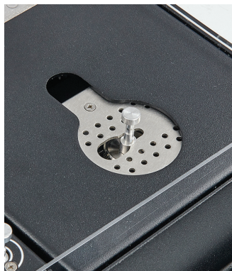
Figure 3: HiSorb probe leak checked, purged and desorbed within the Centri inlet.
