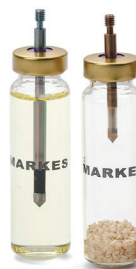
HiSorb probes being used for headspace sampling (right) and immersive sampling (left).
