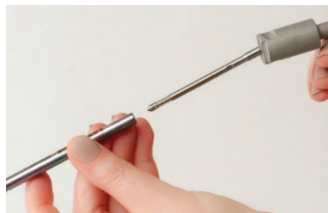
Step [2]: Insertion of the probe into TD tube.
