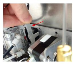
8. Pull the oven down in the direction shown by the red arrow.
