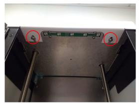
3. Remove the three silver screws (circled in red) from the top of the left-hand side-panel. Pull the panel up and out to remove it.
