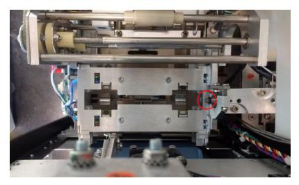
2. Carefully remove the O-ring from the hot nozzle (circled in red), using the O-ring removal tool supplied with the installation kit (shown).
