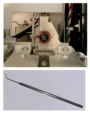
3. Pierce the O-ring with the O-ring removal tool, taking care not to pierce through and scratch the hot nozzle.
