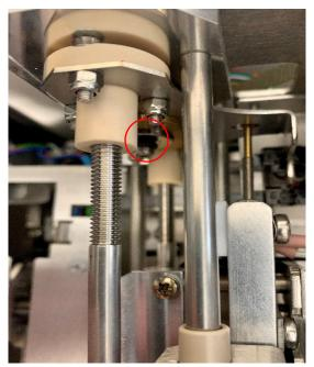
2. Carefully remove the O-ring from the cold nozzle (circled in red), using the O-ring removal tool supplied with the installation kit.
