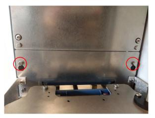
6. Loosen (but do not remove) the nut circled in red, and carefully rotate the cooling fan towards the rear. It may be necessary to tighten the nut circled in yellow, to stop the fan from falling back to its original position.
